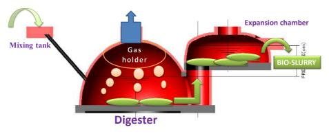
Fig. 11 Bio-slurry production process
