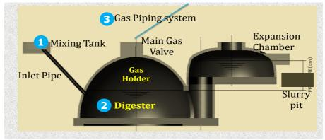
Fig. 1 Modified Biogas plant
