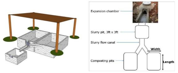
Fig. 14 Bio-slurry management structures
